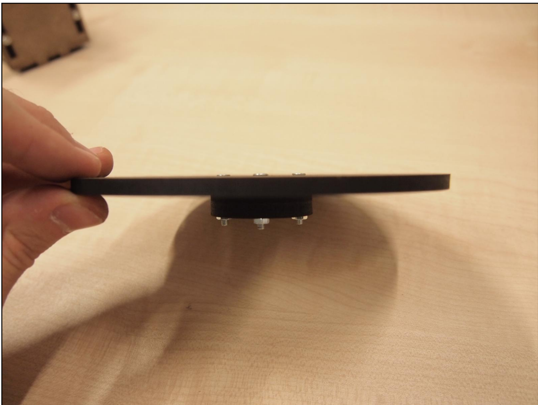
Figure 9: Attach the two small turning table circles to the big turning table using four DIN 965 M3x20 screws and nuts. Make sure the screws are leveled to the surface.
