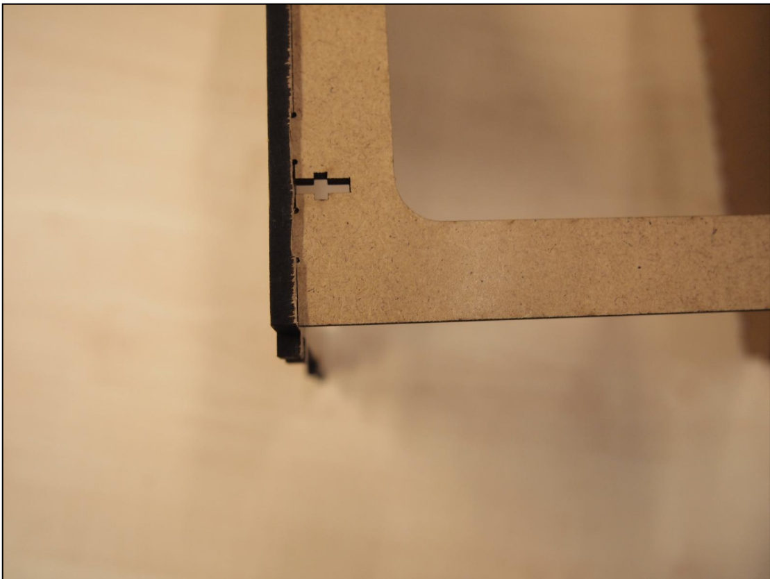
Figure 20: Make sure the box top flush with the Box left or right side. If it doesn't fit you may have mixed up the Box slope and Box top part.
