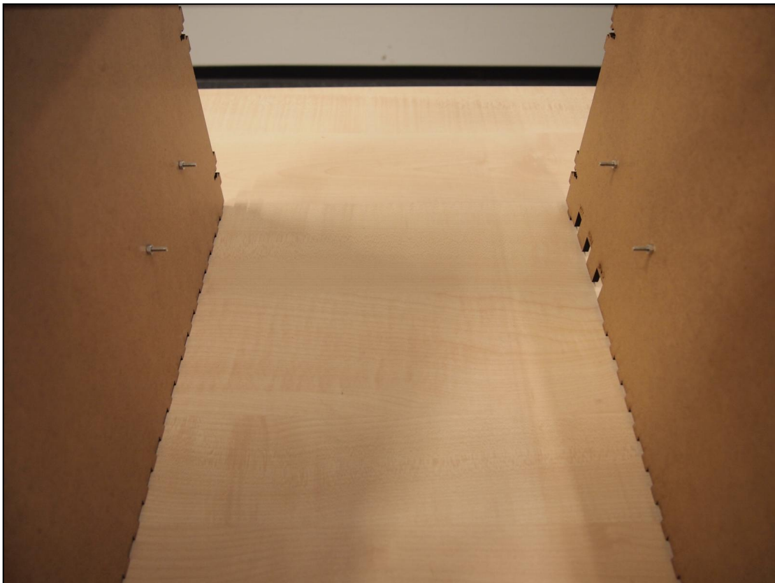
Figure 22: Insert four DIN 912 M3x16 screws and nuts in the holes on the side parts as shown.
